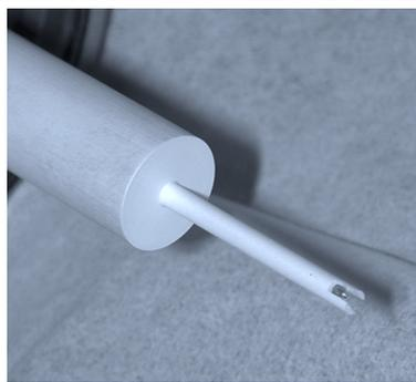
Fig. 3: Photo of baffled probe for HSX.
