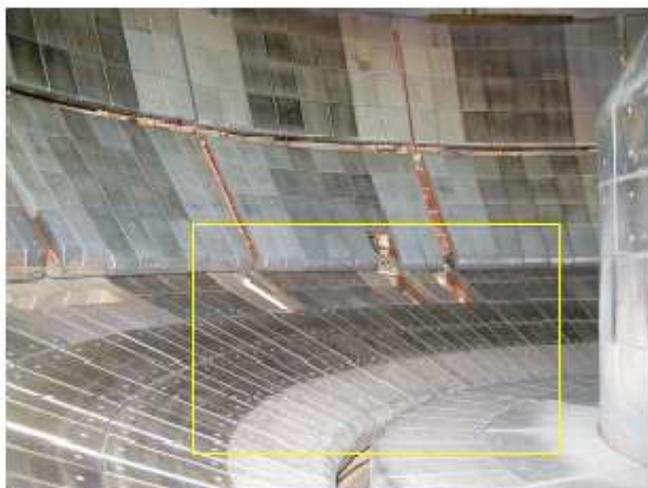
*Fig. 3 – tangential view of the NSTX lower divertor region. The image region of the fast framing visible camera is indicated by the yellow box.*
