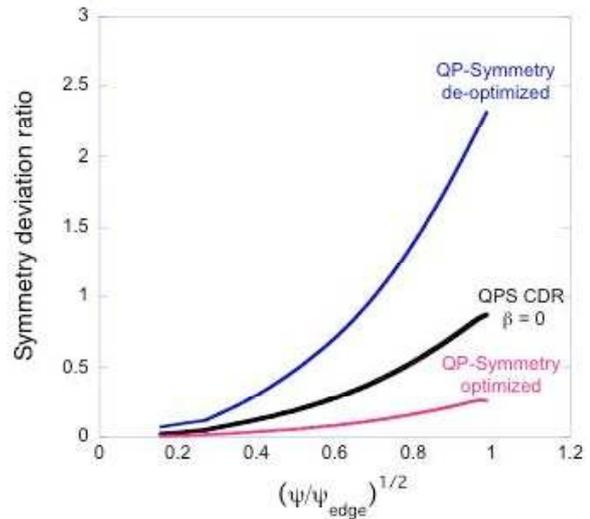
Fig. 5. Changes in the QPS coil currents permit varying degree of (a) neoclassical transport and (b) poloidal symmetry over a wide range.
