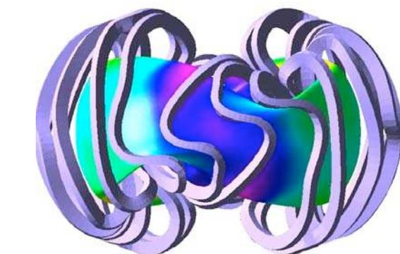
Fig. 2. Top (left) and side (above) views of the QPS plasma and the modular coils used to create it. The colors indicate contours of constant  $|B|(T)$  on the last closed surface.
