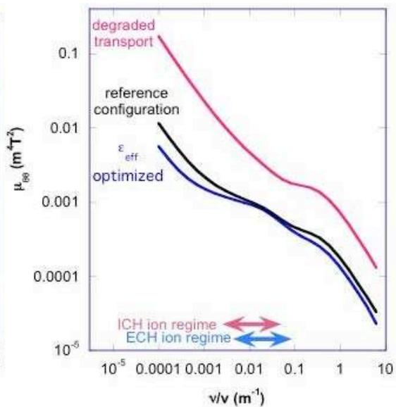
Fig. 7. Variation of poloidal viscosity.
