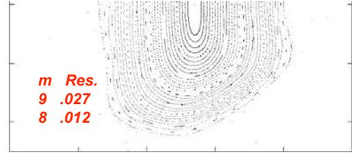
Fig. 4. Varying coil currents reduces magnetic islands in QPS.
