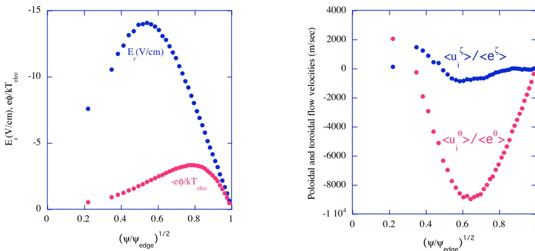
Figure 2 – (a) Ambipolar electric field and potential profiles and (b) poloidal and toroidal flow velocity profiles for QPS ICRF regime parameters.
