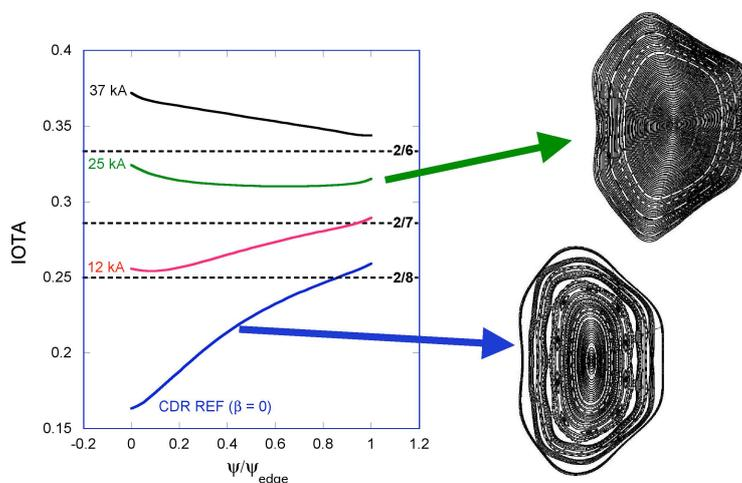
Figure 4 – A range of vacuum  $\dot{\iota}$  profiles produced by variations in coil and plasma currents (labeled to left of the profiles), illustrating good island suppression at 25 kAmps of plasma current.
