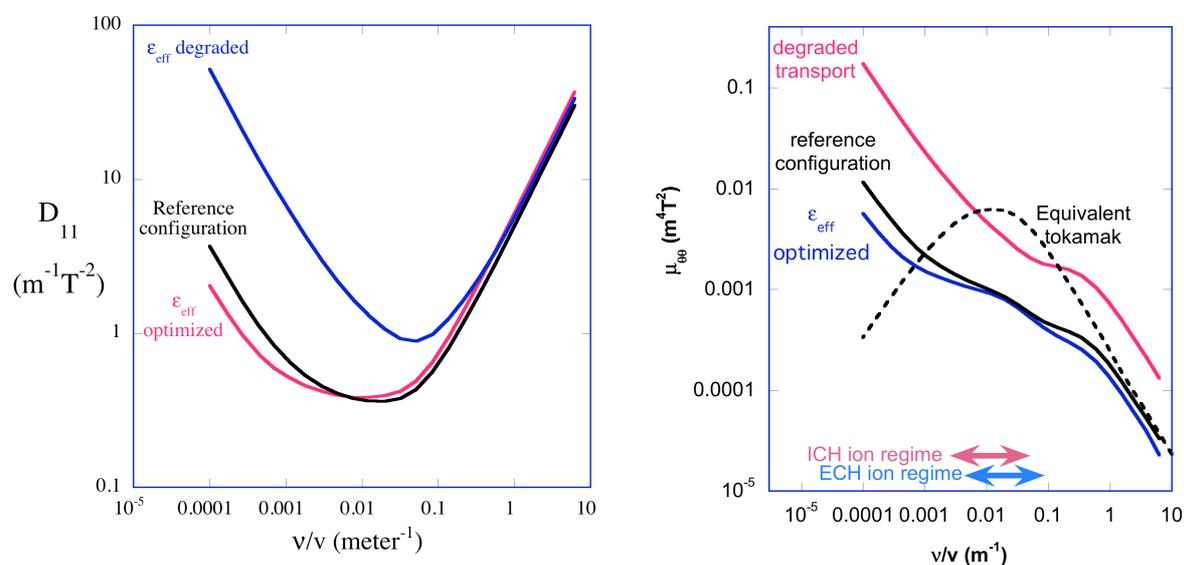
Figure 3 – (a) Monoenergetic transport coefficients vs. collisionality for the reference and transport extremized configurations; (b) Poloidal viscosity coefficient for the reference and transport extremized configurations vs. collisionality. Both plots are for  $\psi = 0.25 \psi_{\text{edge}}$ .
