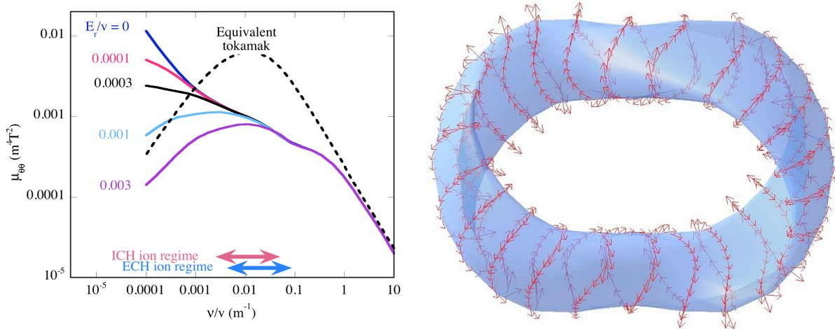
Figure 1 – (a) Poloidal viscosity coefficient at  $(\psi/\psi_{edge})^{1/2} = 0.5$  for quasi-poloidal configuration and equivalent tokamak; (b) Flow velocity vectors and magnetic flux surface at  $\psi/\psi_{edge} = 0.8$  for QPS ICRF regime parameters.
