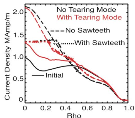
Fig. 4 Comparison of simulated current profile evolution for 3s (to  $t=5.7\text{s}$ ) with (red) and without (black) tearing mode effects where: solid is the initial profile at 2.7s, dashed is the evolved profile including NTM flattening of the temperature profile at  $q \sim 1.5$ , and dotted is the evolved profile with both NTM flattening at  $q \sim 1.5$  and inside the  $q=1$  surface.
