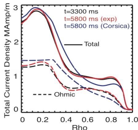
Fig. 2 Simulated and measured total (solid) and Ohmic (dashed) current profiles for DIII-D discharge 117755 conditions with NTM modes present: initial time (black) of 3300ms and those after 2.5s of evolution with observed profiles in red and computed profiles in blue indicating the effect of sawtooth activity on the current profiles.
