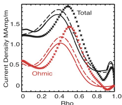
Fig. 1 Comparison of measured and simulated total (black) and Ohmic (red) current profile evolution for a discharge without NTM activity: initial profile (x) and profiles 0.5s later for observed (solid) and computed (dashed) profiles.
