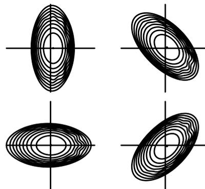
Fig. 2. Poincaré map of the flux surfaces at four cross sections over one field period of a bifurcated LHD equilibrium at  $\beta = 0.04$ . For a broad pressure profile  $p = p_0(1 - s^2)$ , this solution developed a ballooning mode but remained marginally stable.
