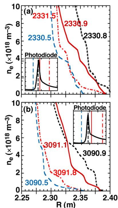
Fig. 2. Edge density profiles during an ELM, at outer gaps of (a)  $4.6 \text{ cm}$  and (b)  $8.3 \text{ cm}$ .
