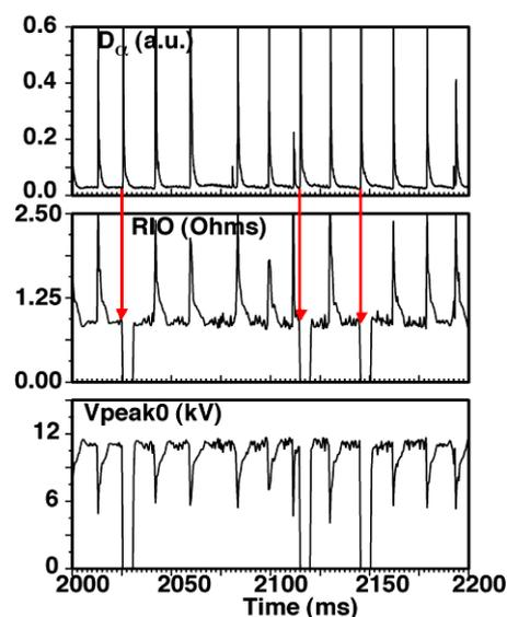
Fig. 3. Arcs triggered by ELMs on the 0 deg array.
