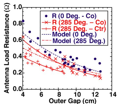
Fig. 1. Series-resonant load resistance for both arrays as a function of outer gap, measured between ELMs.
