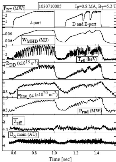
FIGURE 5. Antenna comparison
