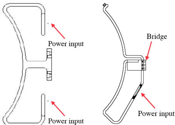
FIGURE 2. Current strap of the 2-strap antenna (left), and the 4-strap antenna (right).
