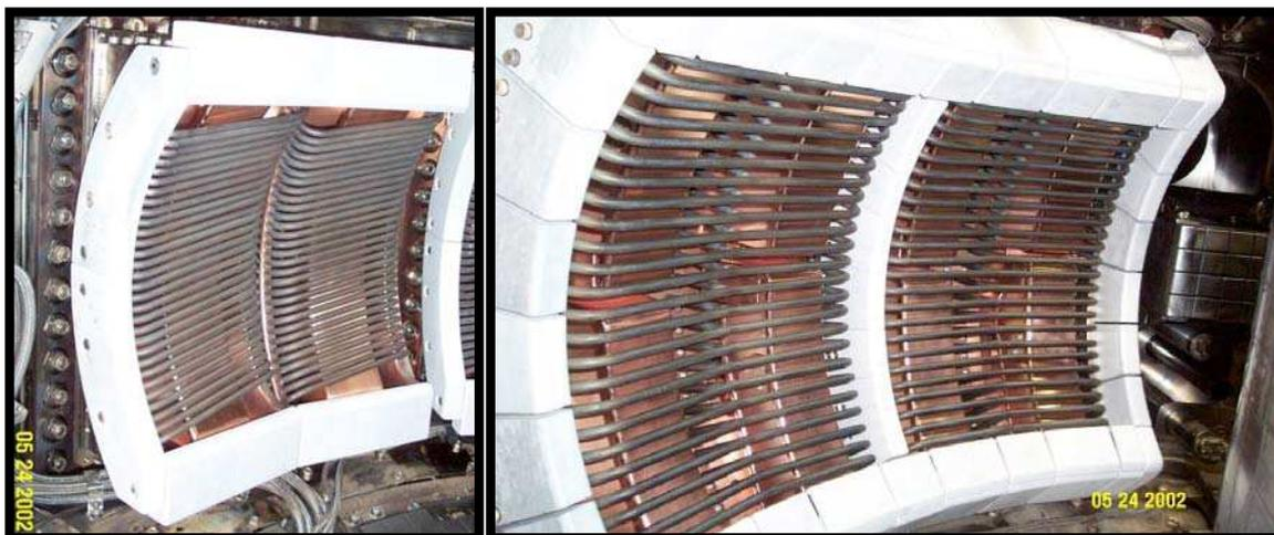
FIGURE 1. One of the two 2-strap antennas (left), and the 4-strap antenna (right).
