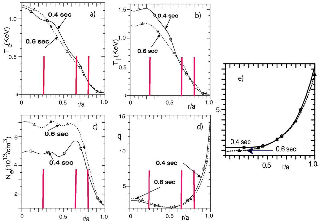
Fig. 1. Profiles from high density H-mode at 0.4 and 0.6 seconds. a) plasma electron temperature, b) ion temperature, c) electron density, d) EFIT derived  $q$  profile, e)  $q$  profile from magnetic diffusion.
