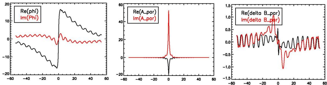
Fig. 2 Real and imaginary components of electrostatic potential and magnetic field eigenfunctions for NSTX H-mode plasma at  $r/a=0.25$  and  $0.6$  sec. Microtearing mode shows tearing parity in  $A_{||}$  component. Mode eigenfunctions shown for seventeen  $2\pi$  field period linear simulations and  $k_{\perp} \rho_s = 0.5$ .
