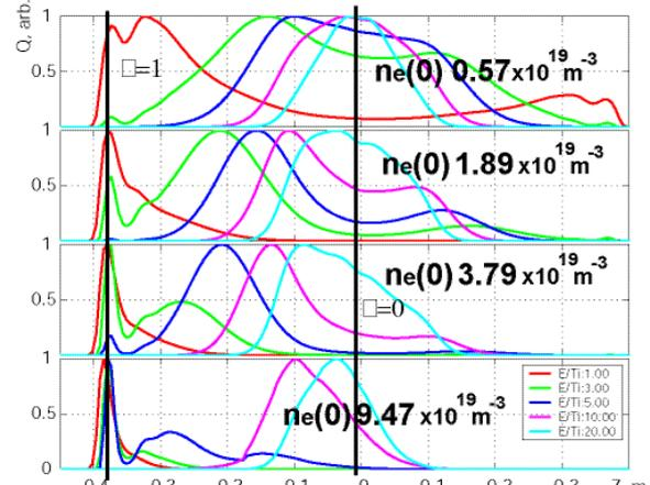
Fig.4: Contribution in CX-spectrum ( $n_a \cdot n_i \cdot f_i \cdot \langle \sigma_{cx}(v_{ia}) \cdot v_{ia} \rangle \cdot \gamma_{att}$ ). Red –  $E=T_i(0)$ ; cyan –  $E=20T_i(0)$ . See fig.3(A) for input profiles.
