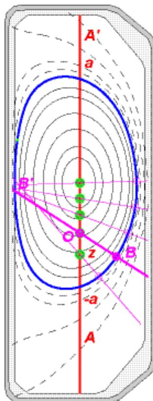
Fig.1: NPA observation geometry. AA' – NPA view line; BB' – chord for 1-D modelling; B – nearest point on plasma boundary for neutral particles calculation in point O.
