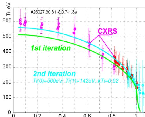
Fig.5: Ion temperature profiles, recovered from NPA measurement and CXRS.
