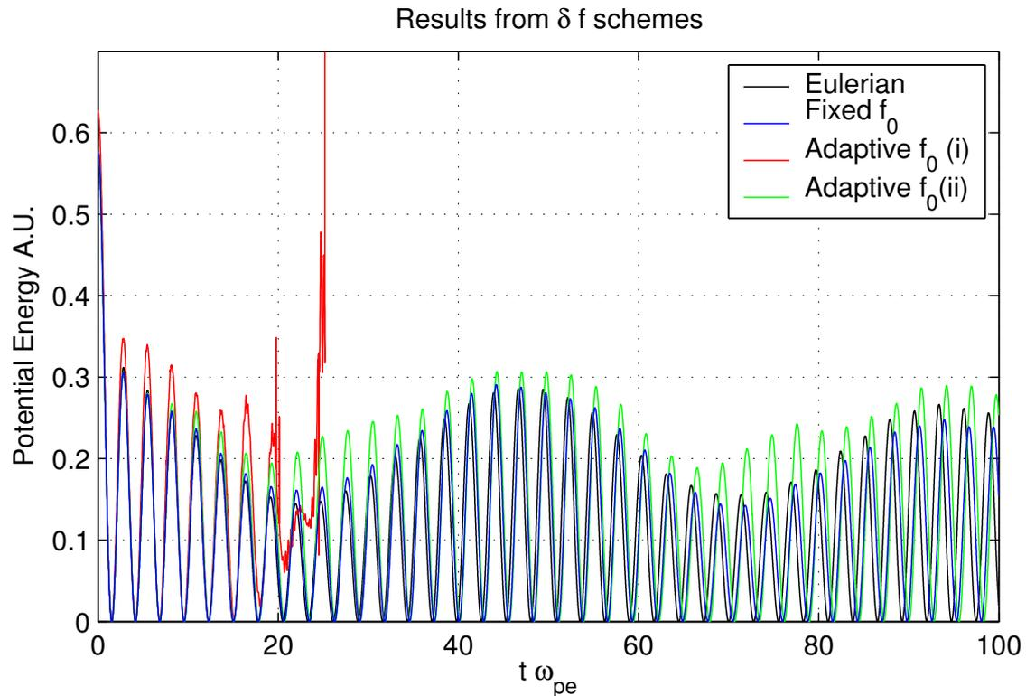
Figure 1: A comparison of the total electrostatic potential energy as a function of time for the Eulerian, fixed  $f_0$  PIC and the two adaptive  $f_0$  PIC variant codes. Algorithm (i) becomes unstable around  $t\omega_{pe} \simeq 23$ .
