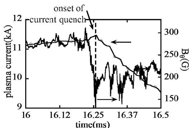
Fig.3 Temporal evolution of inner poloidal magnetic field at inner radial position ( $\rho=0.55$ ).
