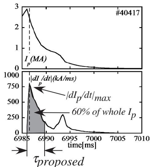
Fig.1 Typical waveform of plasma current and its time differentiation in JT-60U.
