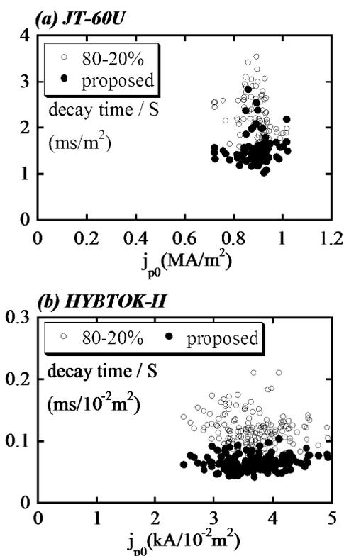
Fig.2 Normalized current quench decay time compared between  $\tau_{80-20}$  and  $\tau_{proposed}$  versus plasma current density before disruption.
