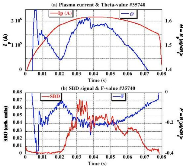
Figure 2. (a): Typical waveforms of the plasma current (red) and of pinch parameter  $\Theta$  (blue). (b): SBD signal at the center chord of vertical array (red) and reversal parameter  $F$  (blue).
