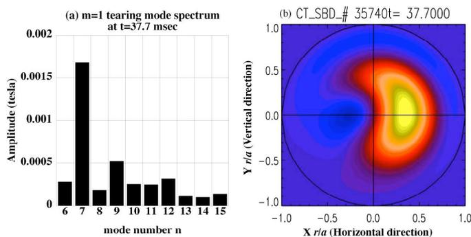
Figure 4. (a): Mode spectrum of  $m=1$  toroidal magnetic fluctuation. The spectrum has a narrow peak at  $n=7$ . (b): Bean shaped hot core.
