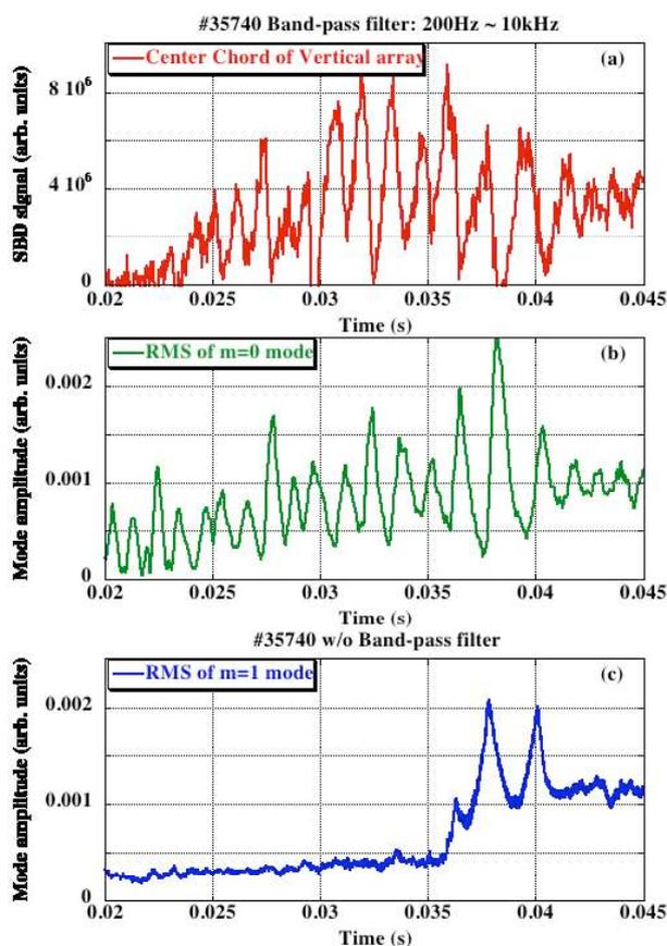
Figure 5. (a): SBD signal with band-pass filter. (b): RMS of  $m=0$  magnetic fluctuation with band-pass filter. (c): RMS of  $m=1$  magnetic fluctuation
