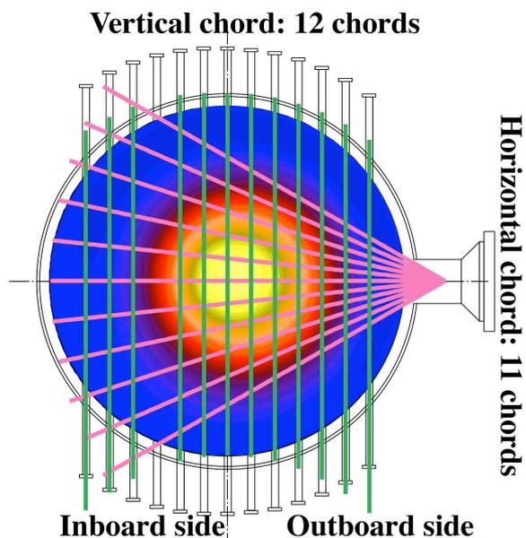
Figure 1. Experimental set up of SBD-CT system. Vertical array consists of twelve SBDs and horizontal array consists of eleven SBDs.
