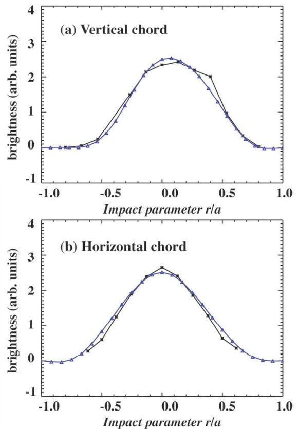
Figure 3. Brightness profiles of vertical chord (a) and horizontal chord (b). Black lines and symbols show the experimental results and blue lines and symbols show the brightness after tomographic inversion.
