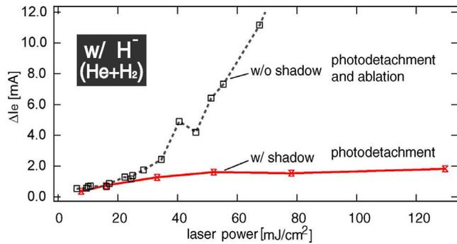
FIG. 2. Laser power dependences of  $\Delta I_e$  with different shadow width.
