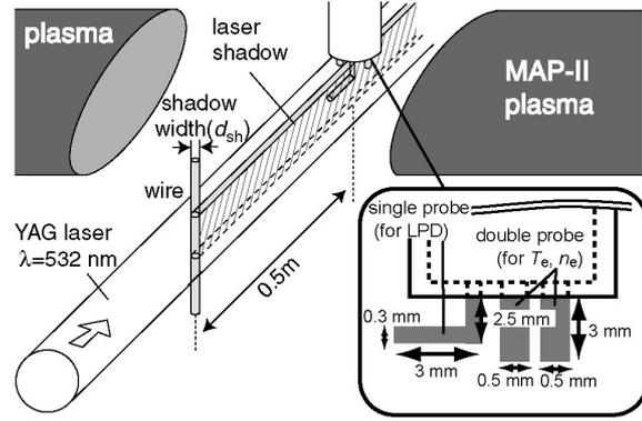
FIG. 1. Schematic of eclipse-LPD arrangement and the probe head: a L-shaped single probe for LPD and a double probe for electron temperature and density measurement.
