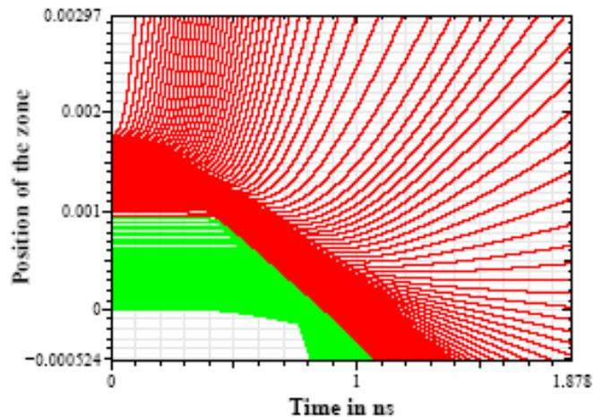
Fig.3. Shock propagation in the aluminium base and carbon step target configuration.
