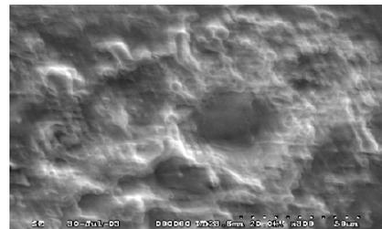
Figure 4: SEM Micrograph ( $\times 800$ ) of laser irradiated copper target, which shows the Surface Boiling and Exfoliation Splashing.
