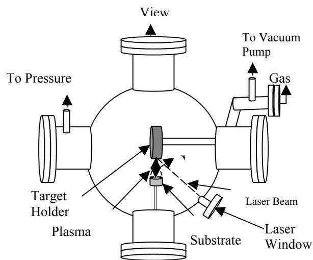
Fig. 1: Schematic of the experimental
