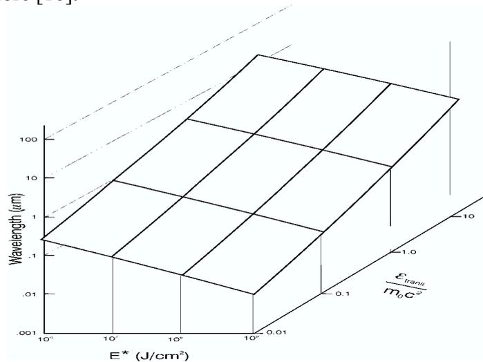
Fig. 3. Relation between the laser wave length the aimed ion energy  $\varepsilon_{trans}$  in multiples of  $m_0c^2$  and the necessary energy flux density for ignition of uncompressed DT following Eq. (3) for  $S = 1$  and a laser pulse length of 3 ps.
