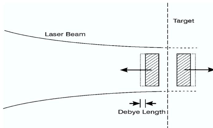
Fig. 2. Scheme of skin depth laser interaction where the non-linear force accelerates a plasma block against the laser light and another block towards the target interior. In front of the blocks are electron clouds of the thickness of the effective Debye lengths of less than 500 nm [13].
