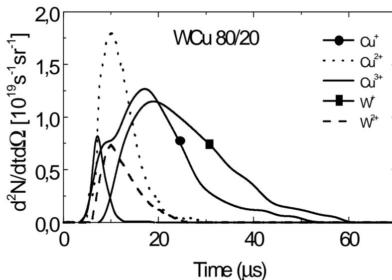
Fig. 1: Time-of-flight spectra of W and Cu ions from the compound system WCu8020.
