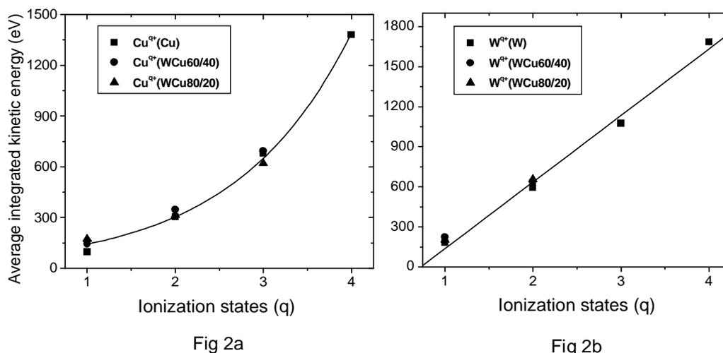
Fig. 2 : Average integrated kinetic energy of copper and tungsten ions from the targets Cu, W, WCu 60/40 and WCu 80/20 as a function of the ionization state.
