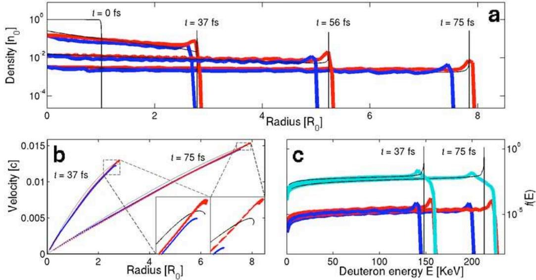
FIG. 2: Evolution of the ion density profile (a),  $v_r - r$  phase space (b), and energy spectrum (c): thin black lines refer to the 1D theoretical model. Red and blue thick lines/dots are used for angular dependent quantities from the simulation results (blue for the  $y$  direction and red for the  $z$  direction, considering the particles contained in a solid angle  $\Omega \approx 0.035$  sr). Cyan lines in (c) represent the total energy spectrum (integrated over the solid angle).
