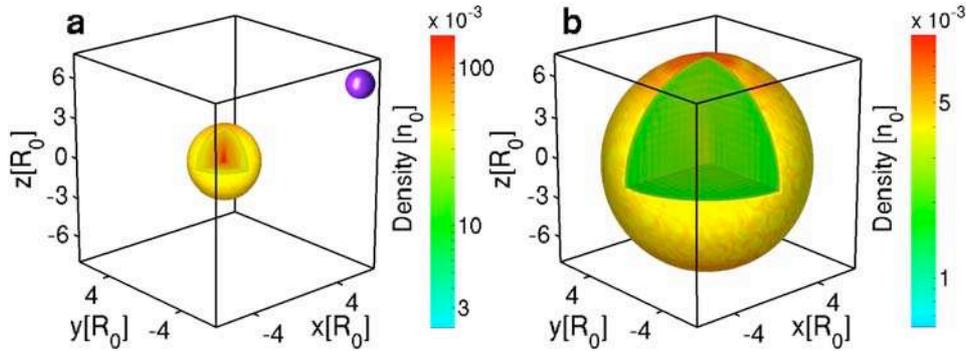
FIG. 1: Ion density distribution in configuration space at time  $t_a = 37 \text{ fs}$  (a), and  $t_b = 75 \text{ fs}$  (b), representing the density variation inside the ion cloud as well as on its outer shell (where the shock front is located). As a reference, a solid sphere having the initial size of the cluster is plotted in (a).
