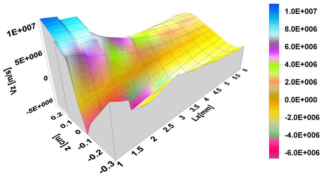
Fig. 2. Ion flow velocity  $V_z$  as a function of dimensions of the acceleration domain.
