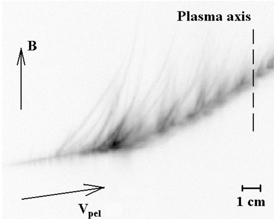
Fig. 1. Integrated photo of the pellet track in shot #41025.
