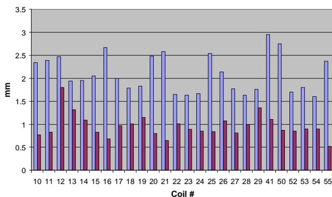
**Fig. 1** Average deviations of already manufactured winding packs. In blue the absolute deviations from the ideal coil shapes and in red the statistical deviations from a mean value of coils of the same type.
