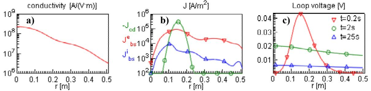
**Figure 2:** a) plasma conductivity; b) the electron ( $\nabla$ ) and ion ( $\Delta$ ) bootstrap current densities, ECCD ( $\circ$ ) density; c) time evolution of the loop voltage.
