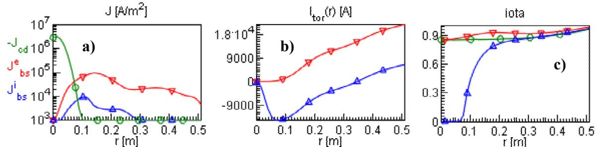
**Figure 4:** a) the electron ( $\nabla$ ) and ion ( $\Delta$ ) bootstrap current densities, ECCD ( $\circ$ ) density; b) the initial ( $\nabla$ ) and final ( $\Delta$ ) toroidal current distributions; c) the initial ( $\nabla$ ), final ( $\Delta$ ), and current free ( $\circ$ ) rotational transform.
