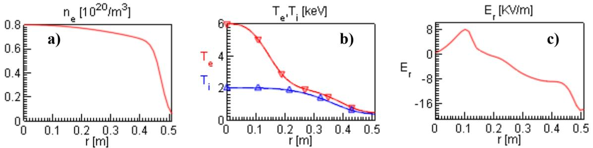
**Figure 1:** Plasma profiles: a) the electron density; b) the electron ( $\nabla$ ) and ion ( $\Delta$ ) temperatures; c) the radial electric field.
