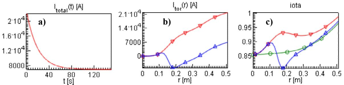
**Figure 3:** a) time evolution of total current; b) the initial ( $\nabla$ ) and final ( $\Delta$ ) toroidal current distributions; c) the initial ( $\nabla$ ), final ( $\Delta$ ), and current free ( $\circ$ ) rotational transform.
