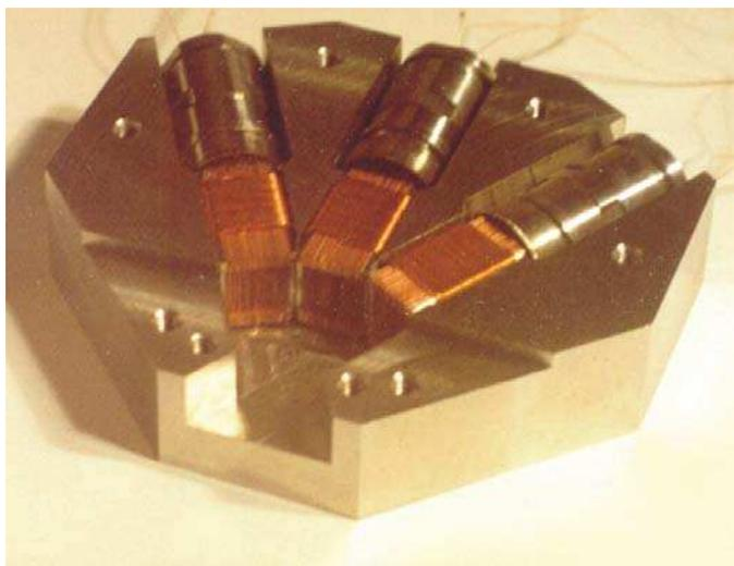
*Fig.1. Photo of pinhole camera of bolometer diagnostics of Globus-M tokamak (cover is removed to show units inside). Every of three collimated channels contains pyroelectric sensor in SS steel case and multislit collimator.*
