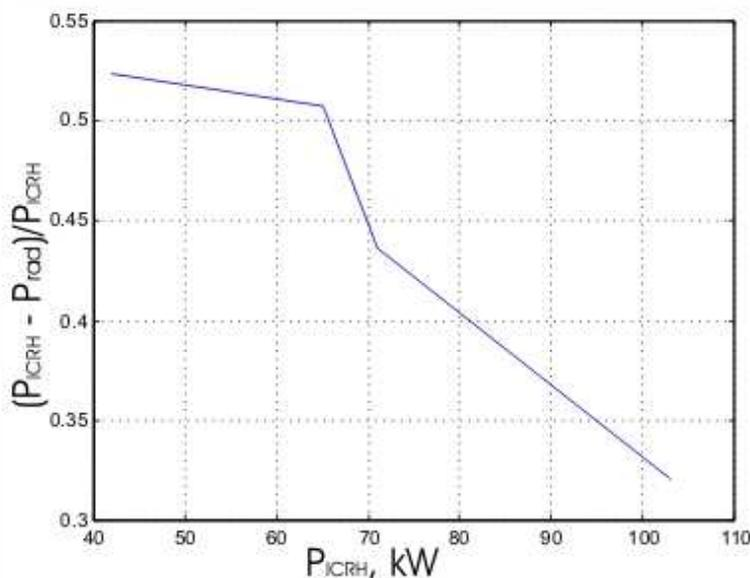
Fig.6. Dependence of ratio of not radiated additional power  $(P_{ICRH} - P_{rad})$  to ICRH power  $P_{ICRH}$  on power source  $P_{ICRH}$ .
