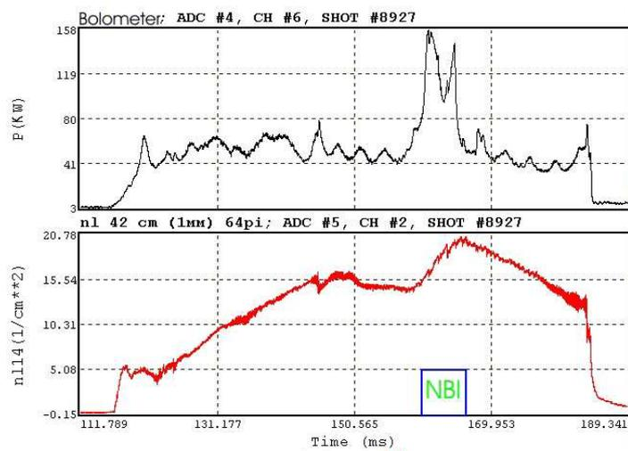
Fig 4. Evolution of radiation losses (upper plot) and central density (bottom plot) in discharge #8927 of Globus-M tokamak with NBI operation.
