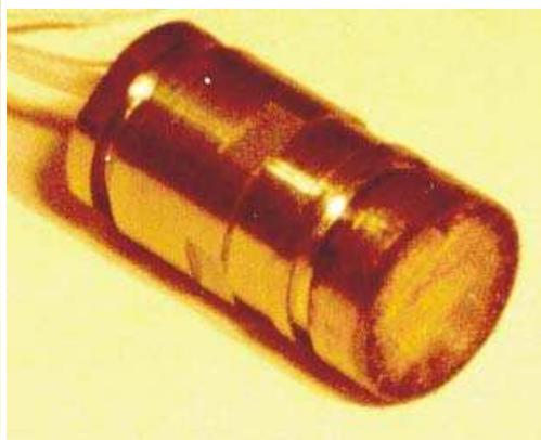
*Fig. 2. Photo of pyroelectric sensor in SS steel case. Face side of the sensor is shielded with a grid.*
