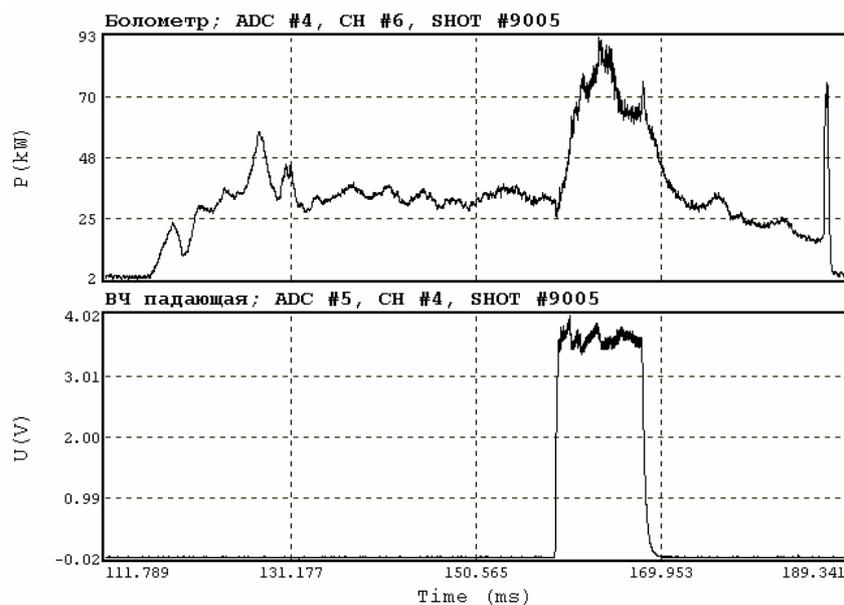
Fig.5 Evolution of radiation losses (upper plot) and ICRH operation (bottom plot) in discharge #9005 of Globus-M tokamak.
