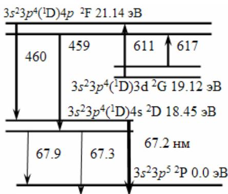
Fig. 1. Diagram of the Ar<sup>+</sup> ion levels involved in the LIF measurements: the 611.5 nm is used for optical pumping, while the 461.0 nm line is used for LIF measurements.
