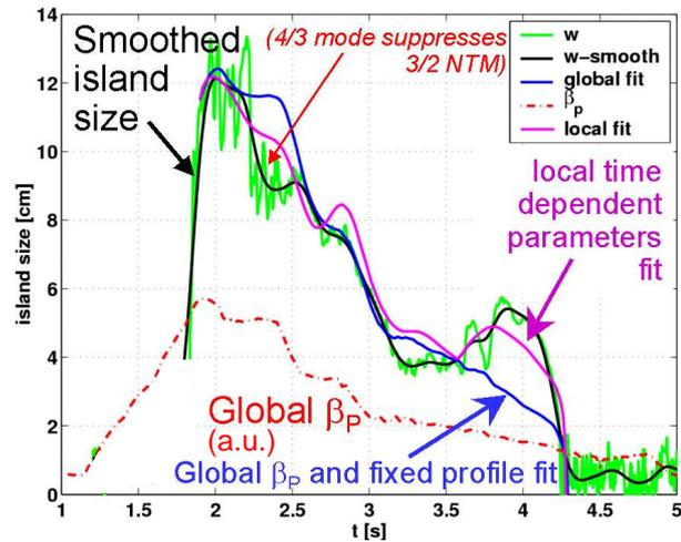
Fig 4: Comparison of different techniques for fitting island evolution for DIII-D shot 111270.
