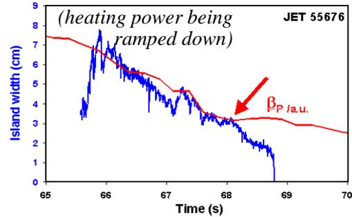
Fig 1: Decoupling of island width (blue) from  $\beta_p$  (red, smooth) at arrowed point as small island size terms start to take effect
