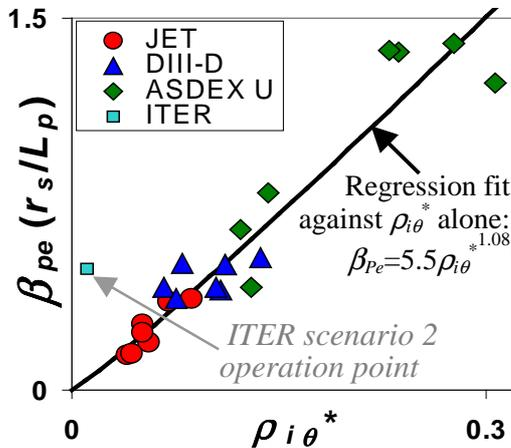
Fig 2: 3/2 NTM metastability threshold scaling plotted against normalised poloidal ion Larmor radius.
