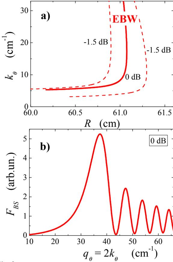
**Fig.2.** (a) Poloidal probing wave number near UHR, (b) BS efficiency for central probing ray.
