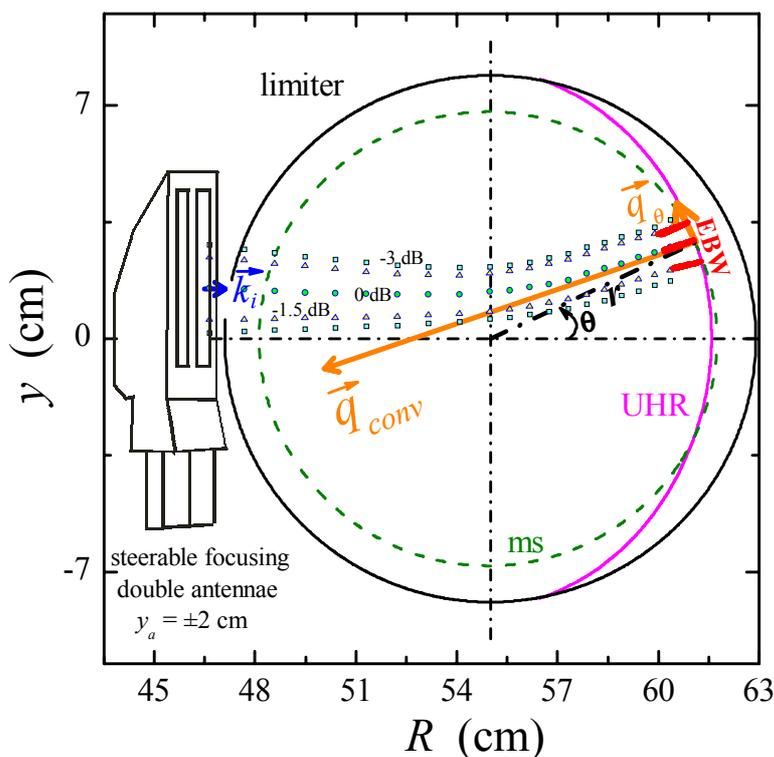
**Fig.1.** Poloidal FT-2 tokamak cross section with antennae set.
