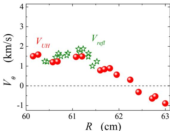
**Fig.4.** Poloidal velocity profiles for  $I_p = 19$  kA. Red circles – UHR BS, green stars – O-mode Doppler reflectometry.
