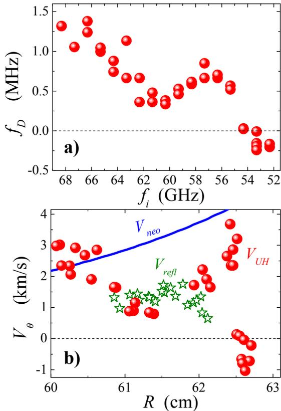
**Fig.3. (a)** Doppler frequency shift versus incident frequency ( $y_a = +15$  mm).
