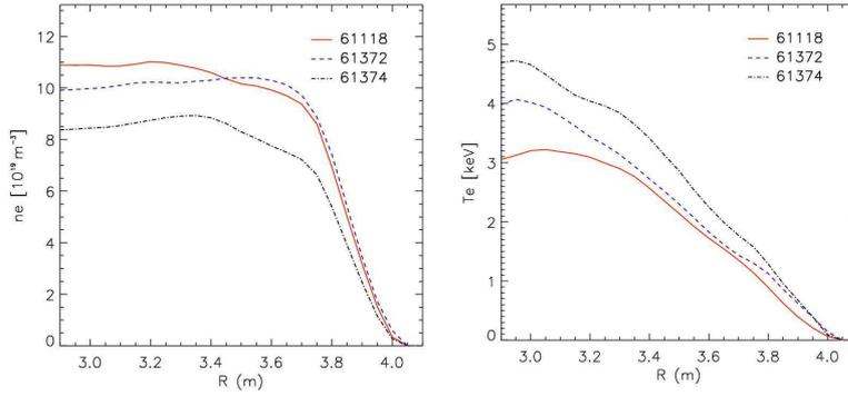
Figure 2: Electron density and temperature from LID R diagnostic averaged between the start of tritium puff and 500 ms later for the three pulses, #611374, #61372 and #61118.
