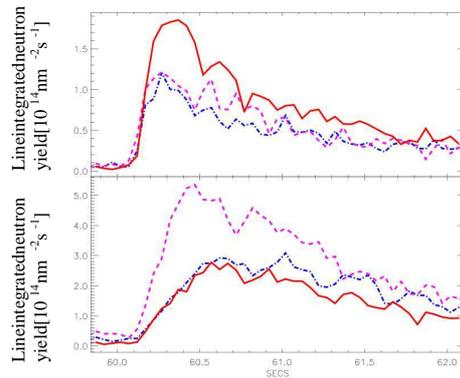
Figure 3: Time traces of the 2 horizontal camera channels. Edge channel number 1 (top figure), and core channel number 4 (bottom figure), for the pulses #61118 (red continuous line), #61372 (blue dash dotted line) and #61374 (magenta dashed line)
