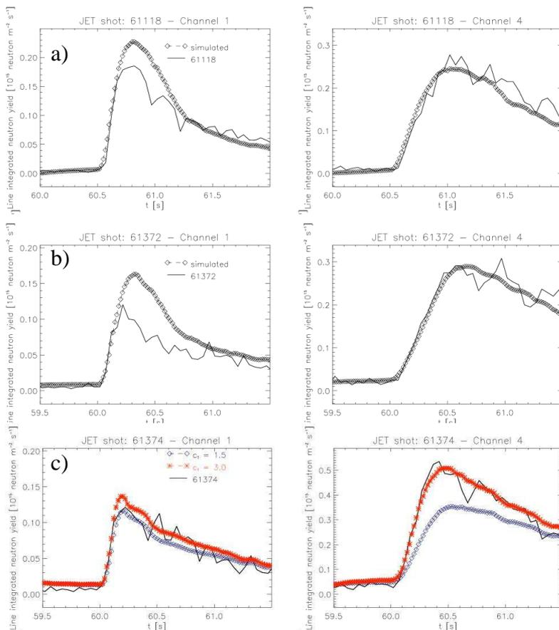
Figure 4: Experimental and simulated neutron line average emissivity for an edge channel 1 (left) and central channel 4 (right) for the three pulses: #61118, #61372 and #61374
