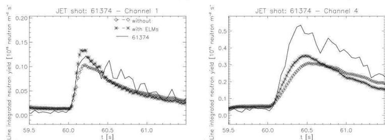
Figure 6: Experimental and simulated neutron line average emissivity for an edge channel 1 (left) and central channel 4 (right) for shot #61374. The simulated results are for two extreme cases without ELMs and with the highest ELM frequency.
