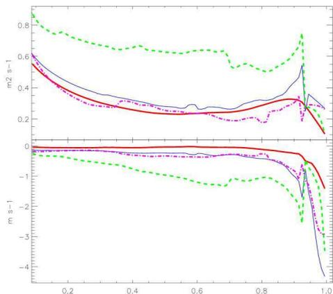
Figure 5: Tritium diffusion (top) and convective velocity (bottom) for the pulses #61118 (red neo-classical, blue neo-classical plus anomalous, continuous line), #61372 (magenta dashed and dotted line) and #61374 (green dashed line)
