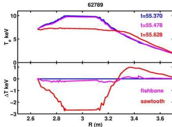
Figure 5. Profile modification by a fishbone (magenta) and by an ordinary sawtooth (red).
