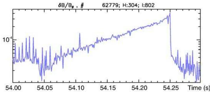
Figure 3. Amplitude of magnetic oscillations during a slow sawtooth cycle in lin-log scale. The  $e$ -folding time is 90 ms.
