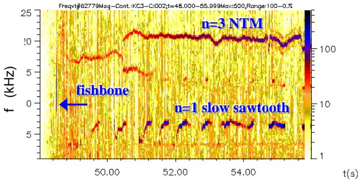
Figure 2. Spectrogram of magnetic oscillations below 25 kHz. Bursts between 4 and 7 kHz are  $n=1$  slow sawteeth. The line near 20 kHz is an  $n=3$  NTM. The intense, almost vertical line at  $t=48.6$  s is a fishbone.
