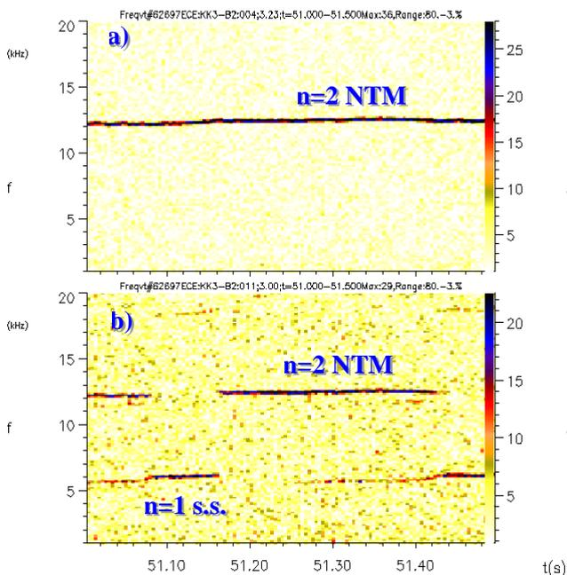
Figure 7. ECE spectrograms. a)  $R= 3.26$  m showing the  $3/2$  NTM at 12 kHz. b)  $R=3$  m showing the slow sawtooth at 6 kHz and the NTM expulsion from the central region at  $t=51.08$  and  $51.43$  s.
