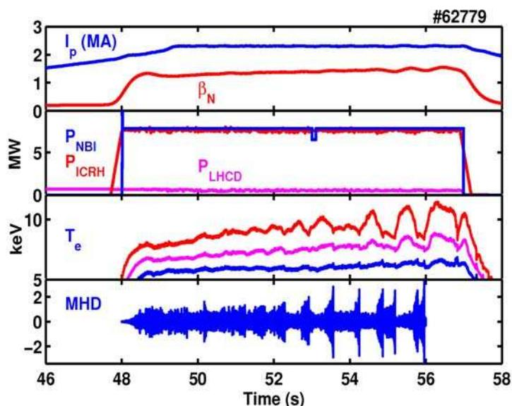
Figure 1. Time traces of a hybrid JET discharge with  $B=3.2T$ ,  $I=2.3MA$  and dominant electron heating ( $T_i \approx 0.6T_e$ ).  $T_e$  traces are given at  $R=3.15m$  (red),  $3.225m$  (magenta) and  $3.3m$  (blue). MHD trace gives edge poloidal field oscillations between 2 and 10 kHz.
