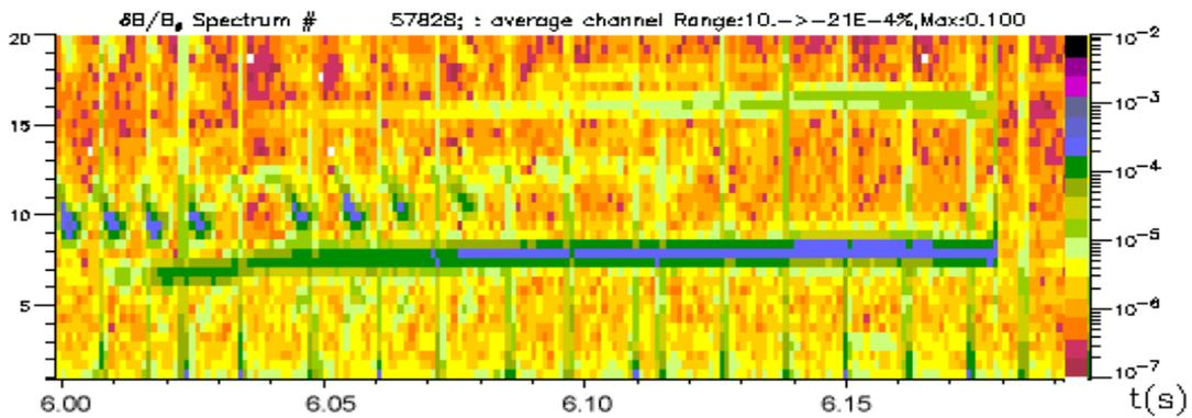
Figure 6. Spectrogram showing a direct comparison between a slow sawtooth (line below 8 kHz) and fishbones (modes with frequency chirp between 12 and 9 kHz). The line at 16 kHz is the  $m=2$  second harmonic of the slow sawtooth.
