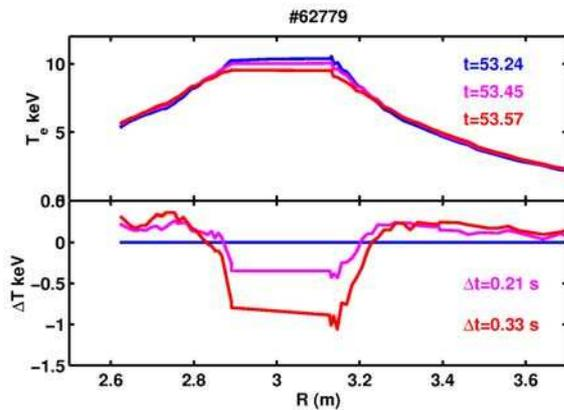
Figure 4. Profile evolution during a slow sawtooth. Red traces are at the top of mode amplitude.
