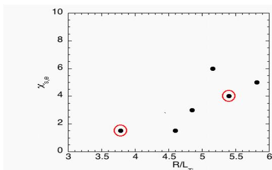
*Fig.1: Experimentally determined trend of the amount of electron stiffness versus the ion temperature inverse gradient length. The two encircled shots are the ones chosen for the detailed predictive modelling with various transport models.*
