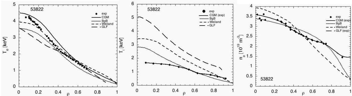
Fig.2: Steady-state experimental profiles of  $T_e$ ,  $T_i$  and  $n_e$  for shot 53822 (dots) and simulations using various models: : empirical CGM (—), Weiland with collisions (---), Bohm-gyroBohm (.....) and GLF23(— · —).
