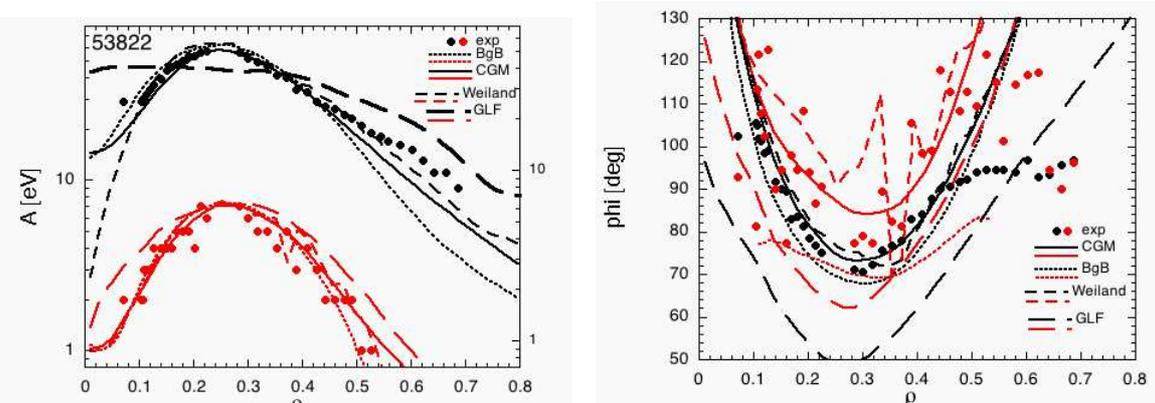
Fig.4: Experimental profiles (dots) of amplitude and phase at 1<sup>st</sup> (black) and 3<sup>rd</sup> (red) harmonic for shot 53822 and simulations using various models: empirical CGM (—), Weiland with collisions (---), Bohm-gyroBohm (.....) and GLF23(— · —).
