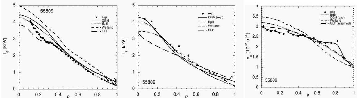
Fig.3: Steady-state experimental profiles of  $T_e$ ,  $T_i$  and  $n_e$  for shot 55809 (dots) and simulations using various models: : empirical CGM (—), Weiland with collisions (---), Bohm-gyroBohm (.....) and GLF23(— · —).
