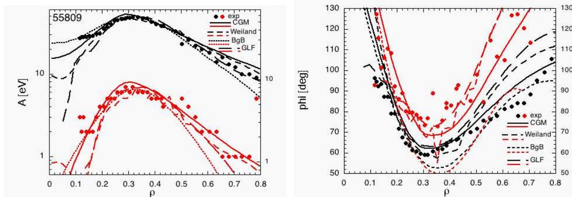
Fig.5: Experimental profiles (dots) of amplitude and phase at 1<sup>st</sup> (black) and 3<sup>rd</sup> (red) harmonic for shot 55809 and simulations using various models: empirical CGM (—), Weiland with collisions (---), Bohm-gyroBohm (.....) and GLF23 (- - -).
