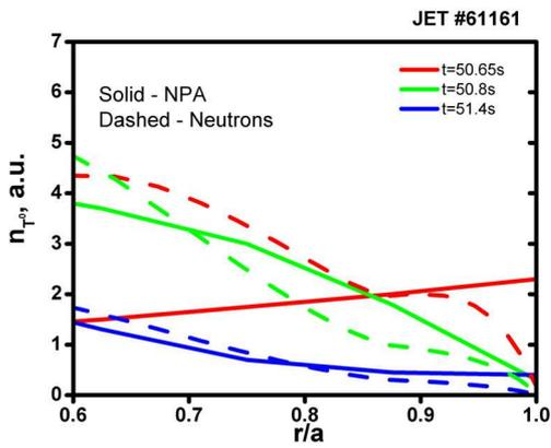
Fig.3 Comparison of tritium profile evolution obtained from NPA and neutron data.
