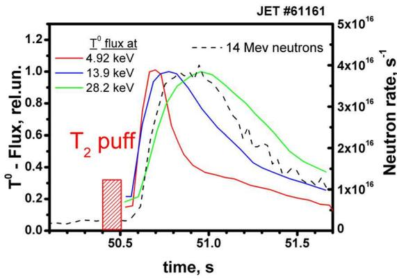
Fig.1 ISEP NPA and 14 MeV neutrons traces. Tritium gas puff in JET shot #61161.
