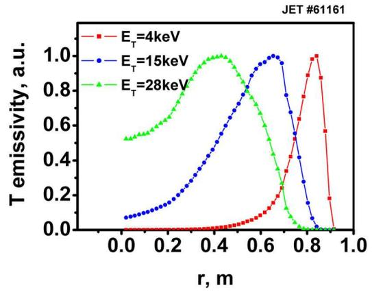
Fig.2 Source functions for tritium neutral fluxes of different energies.
