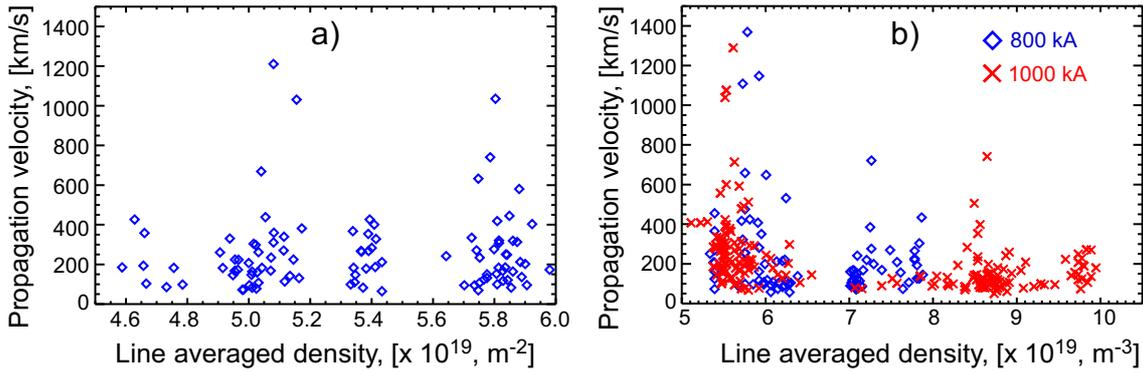
Figure 2: Velocities of propagation of the ELM perturbation as measured by ICRF antennas, depending on central line averaged densities for JET (a) and ASDEX Upgrade (b).
