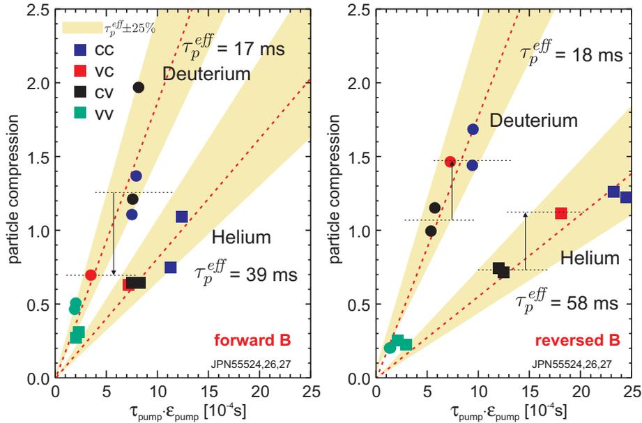
Figure 3: Particle compression for helium and deuterium as a function of the pumping efficiency multiplied by the characteristic pumping time.
