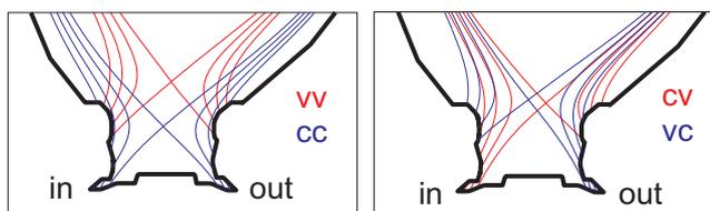
Figure 1: The four configurations of the strike point positions (e.g. **vc** means inner strike point at the vertical target and outer strike point at the corner position).
