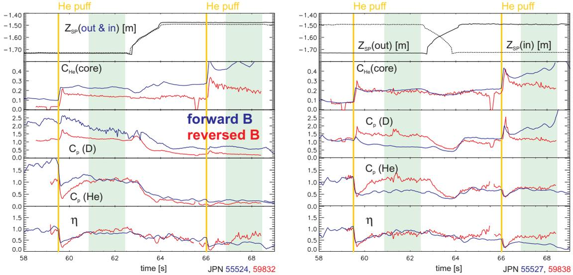
Figure 2: Typical time traces of the strike point position, the helium concentration, the pumping efficiency, the compression and the helium enrichment. The lefthand figure shows the symmetric strike point configurations (*cc* and *vv*), the righthand figure shows the asymmetric configurations (*vc* and *cv*). The relevant flat-top regions are marked with the green boxes.
