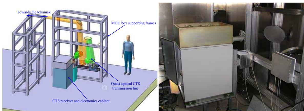
Figure 3: Left: Illustration of the transmission line for ASDEX-Upgrade. Right: The CTS system installed at ASDEX Upgrade, with the moveable mirror to the right.
