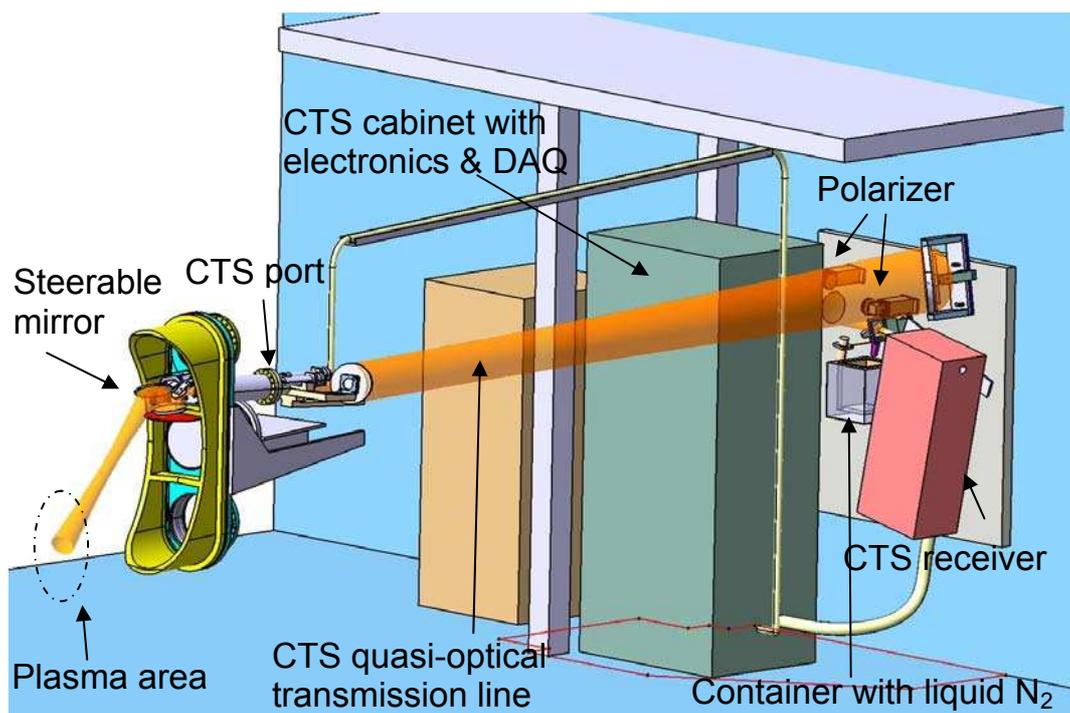
Figure 2: The upgraded quasi-optical transmission line for TEXTOR.
