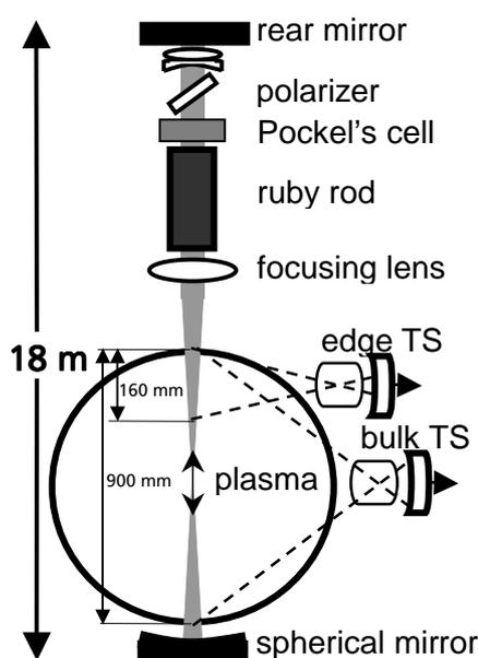
Fig 1. Schematic of the intra-cavity ruby laser at TEXTOR. The viewing lenses for bulk and edge measuring chords are also shown.
