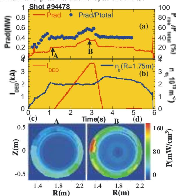
Figure 1 The time trace of (a) the total radiation power (red), the ratio of the total radiation power over the total input power (closed circle); (b) the line-averaged central density (blue) and current of DED coil #1 measured in the plasma with DC. (c) and (d) show the 2-D radiation profiles at 1.1s and 2.9s, respectively.
