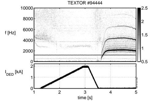
Figure 2: Spectrogram of a magnetic pick-up coil (top), and DED coil current (bottom). The  $2/1$  tearing mode excited by the error field is locked and starts rotating when the external field is switched off.
