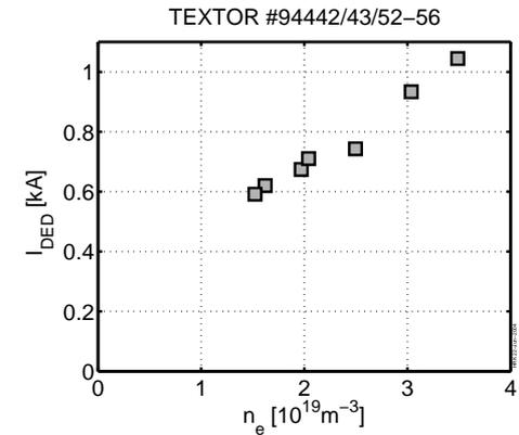
Figure 3: Critical DED coil current at mode onset versus the line-averaged electron density.
