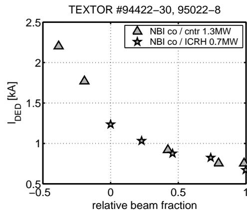
Figure 5: Critical DED current versus the relative fraction of co and counter neutral beam heating.
