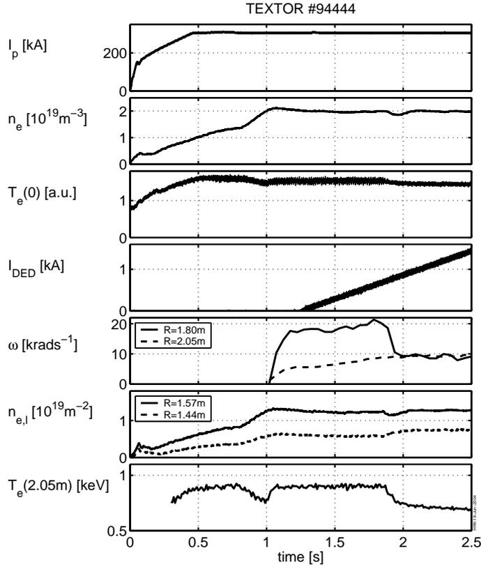
Figure 1: Time traces of various signals showing the time evolution of an experiment with slow DED ramp-up in dc mode. The signals from top to bottom are: plasma current, line-averaged electron density, central electron temperature, DED coil current, toroidal plasma rotation frequency (core and edge), two line-integrated electron density measurements close to the  $q = 2$  surface, and the electron temperature at the  $q = 2$  surface.
