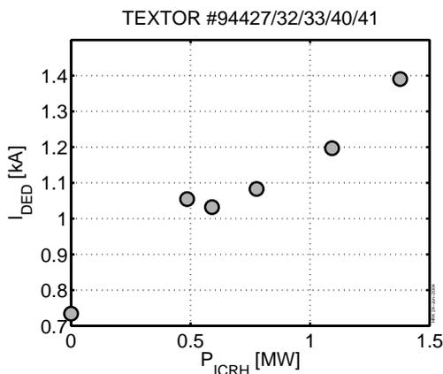
Figure 4: Increase of the threshold for mode onset with ICRH heating power.
