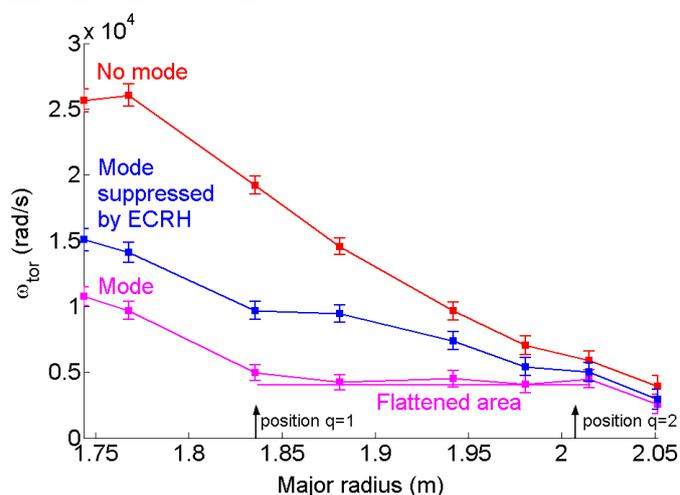
**Figure 4:** Rotation profiles before the mode, during the mode and during mode suppression by ECRH. When the mode is present a large area of the rotation profile, extending from the position of  $q=2$  to  $q=1$ , is flat.
