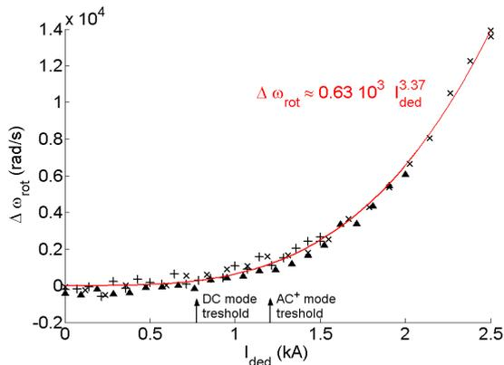
**Figure 2** The increase in rotation plotted against the DED current. A fit to the data with a monotonic increasing function shows approximately a cubic relation. (the different symbols represent different plasma discharges)
