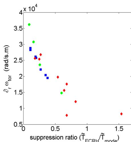
**Figure 5:** The gradient of the rotation profile plotted against the suppression ratio determined from ECE signals. The green circles are data from an ECRH power scan, the blue squares from a phase scan (relative to the DED) and the red diamonds from a deposition radius scan.
