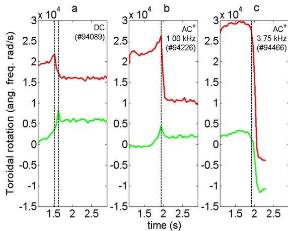
**Figure 3** The effect of mode excitation on the central rotation (red trace  $R = 1.74\text{m}$ ) and on the rotation more towards the edge (green trace  $R = 2.0\text{m}$ ).
