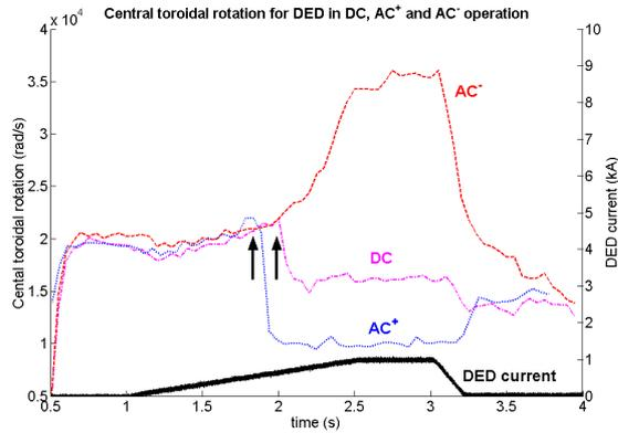
**Figure 1** Increase in rotation is seen in DC, AC<sup>+</sup> and AC<sup>-</sup> operation. For DC and AC<sup>+</sup> operation mode excitation occurs which breaks down the rotation (black arrows), for AC<sup>-</sup> excitation of the 2/1 mode is avoided and the rotation increases as long as the DED current increases (and decreases when de DED current decreases again)
