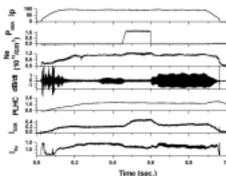
Fig.1 Suppression of MHD instability by 24MHz IBW wave ( $I_p=157.6kA$ ,  $B_t=1.76T$ ,  $P_{IBW}=156kW$ ,  $q_a=3.1$ , the IBW  $\Omega_H$  or  $2\Omega_D$  ion cyclotron resonant layer is located near 0.5a)
