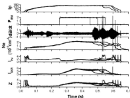
Fig.2 Suppression of MHD instability by 30MHz IBW wave ( $I_p=168kA$ ,  $B_t=1.99T$ ,  $q_a=3.2$ ,  $P_{IBW}=195kW$ , the IBW  $\Omega_H$  or  $2\Omega_D$  ion cyclotron resonant layer is located in the plasma centre).
