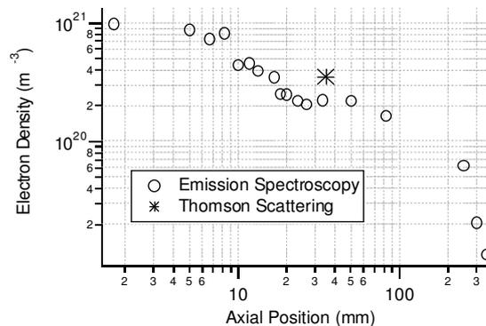
Fig. 5: The axial variation of electron density on a double logarithmic scale as measured with HR OES at 0.4 T.
