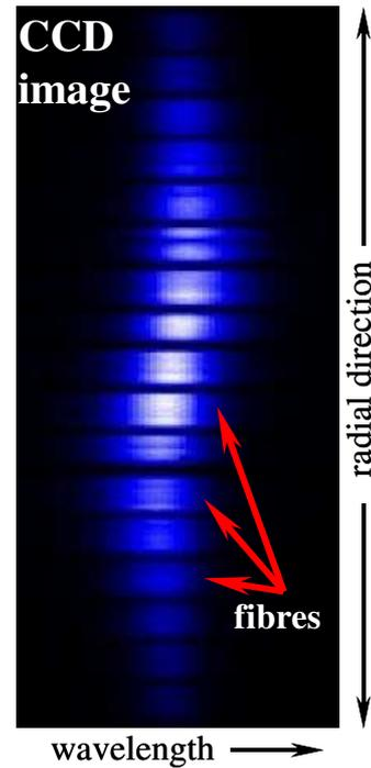
Fig. 3: H<sub>β</sub>-line emitted across the plasma jet. The light from separate fibres is
