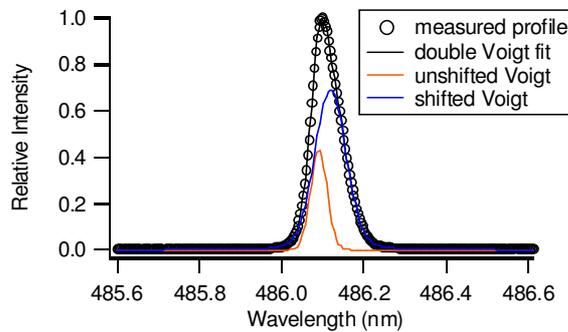
Fig. 4: Asymmetric profile of H<sub>β</sub>-line and two Voigt components of the fit.
