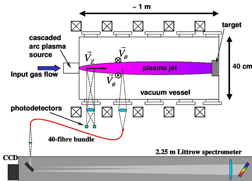
**Fig. 1:** Schematic drawing of the Pilot-psi linear plasma generator and the optical system for high-resolution emission spectroscopy.
