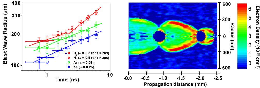
Figure 2. (a) Measured blast wave trajectories for H, Ar and Xe cluster media. Solid lines represent the best fit to the data. (b) Electron density map of a tailored blast wave in a H cluster medium after 6 ns.
