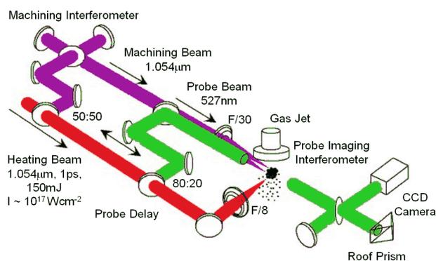
Figure 1. Experimental layout for producing tailored blast waves in an atomic cluster medium.
