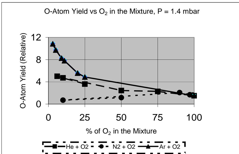
Fig.1: Yield of O-atoms with different compositions of Ar-O<sub>2</sub>, He-O<sub>2</sub> and N<sub>2</sub>-O<sub>2</sub> gas mixtures as a function of O<sub>2</sub> fraction.
