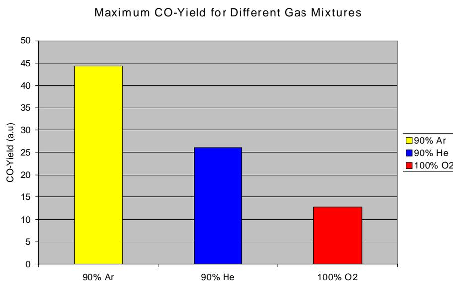
Fig. 2: Bar graph showing the maximum yield of CO for different gas mixtures but at low pressures around 0.3 mbar.
