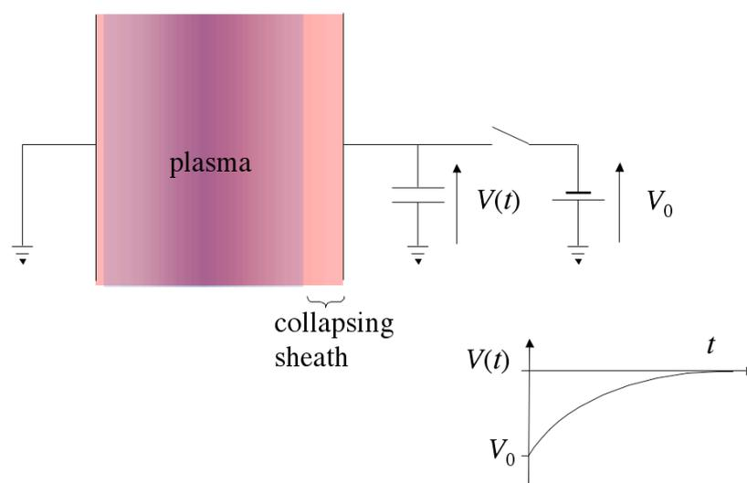
Figure 1 Schematic showing the situation that is being modelled
