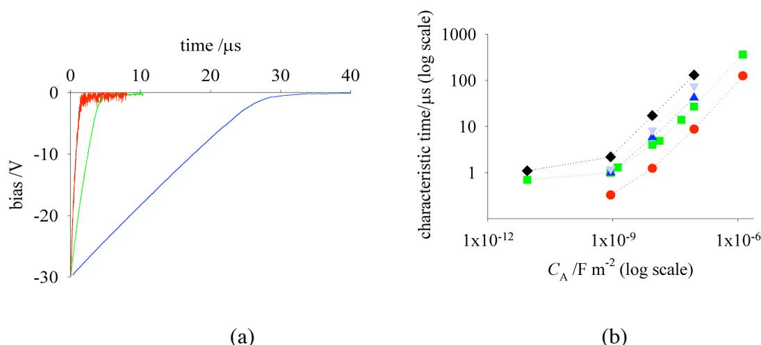
**Figure 2 (a)  $V(t)$  for  $C_A = 8.8 \times 10^{-8}$  (Blue);  $8.8 \times 10^{-9}$  (Green) and  $8.8 \times 10^{-10}$  (Red) F m<sup>-2</sup> (b) characteristic times for  $V_0=10$ (circle), 30(square), 50(up-triangle), 100(down-triangle) and 200(diamond) V against  $C_A$ .**
