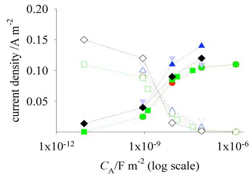
**Figure 3 External current (open symbols) and displacement current (closed symbols) at the surface of the RH electrode for  $V_0=10$ (circle), 30(square), 50(up-triangle), 100(down-triangle) and 200(diamond) V.**
