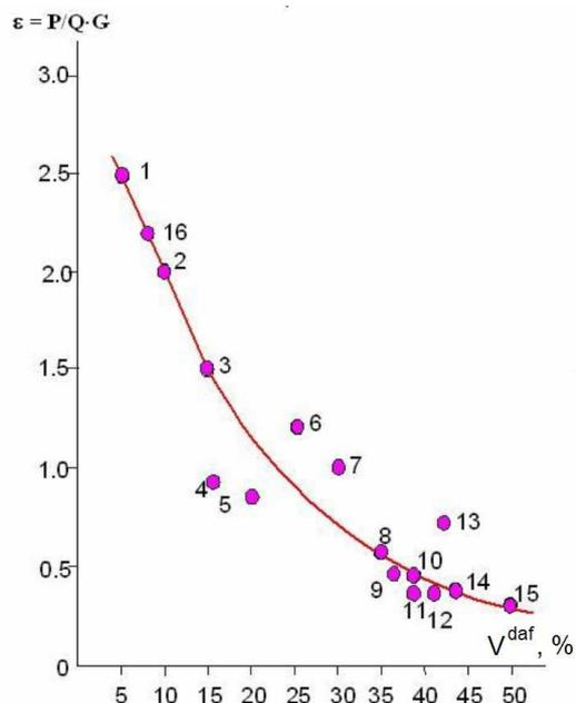
Figure 5. Experimental dependence of relative electric consumption of a plasmatron from a yield of ignited coal volatiles at different thermal power plants: 1 – Northern Korea; 2, 12 – Ukraine; 3 –
