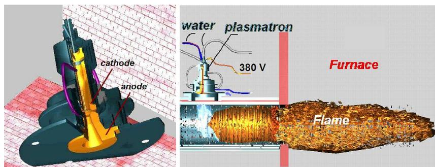
Figure 2. Plasmatron and scheme of its mounting onto direct flow pulverized coal burner.
