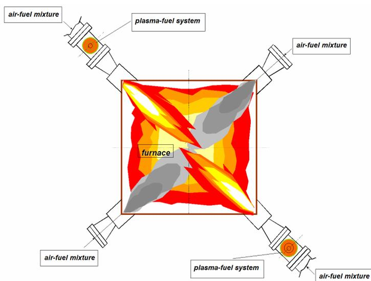
Figure 3. Diagram of mounting of burners onto the boiler with 420 t/h steam productivity equipped with the plasma-fuel systems ignition the air-fuel mixture at the Ulan-Bator thermal power plant 4 (Mongolia).
