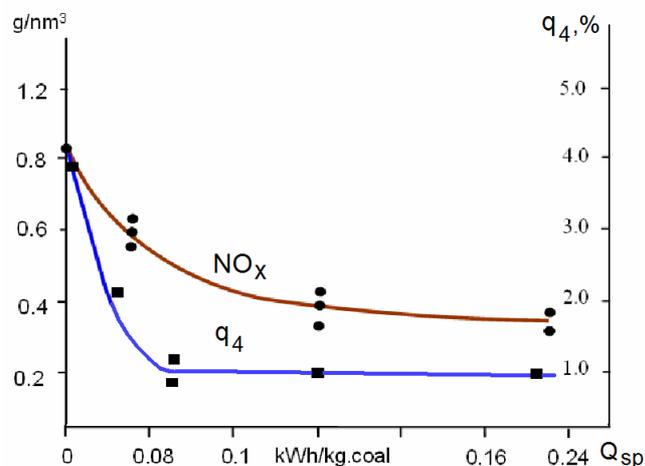
Figure 4. Reduction  $NO_x$  formation and unburned carbon ( $q_4$ ) versus specific energy consumption ( $Q_{SP}$ ) for plasmatron.
