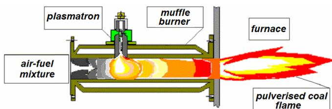
Fig. 1. Plasmatron and scheme of its mounting onto direct flow pulverized coal burner (plasma-fuel system) and the furnace chamber dividing for finite volumes scheme.
