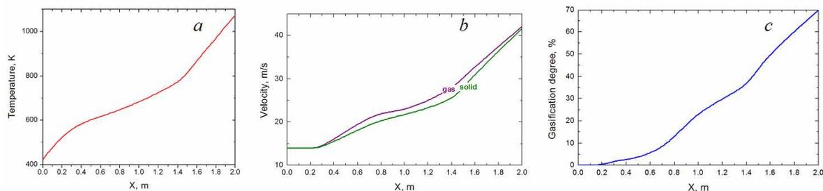
Fig. 2 Temperature of the products along the PFS (a); velocity of the products along the PFS (b); coal gasification degree variation along the PFS (c).
