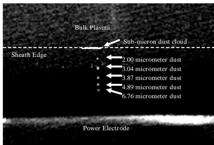
Figure 3 Levitation of sub-micrometer particle used in the determination of sheath width
