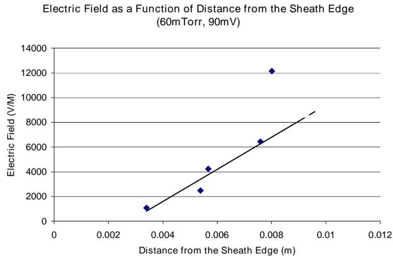
Figure 3 Graphs showing the electric fields calculated at various heights of the sheath
