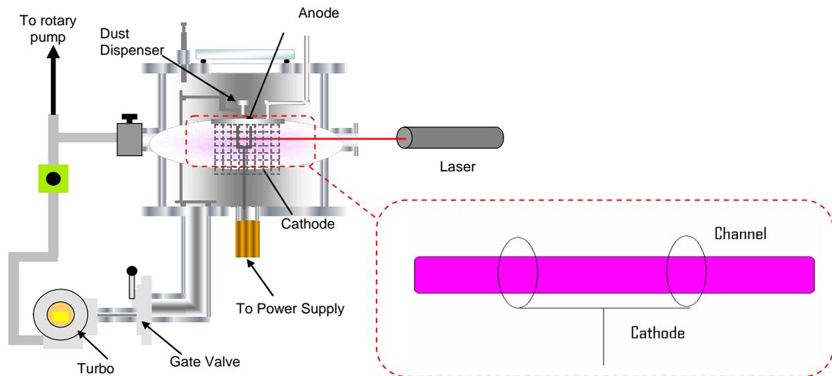
Figure 1. Schematic diagram of setup (on the insert the schematic diagram of cathode and ion channel)
