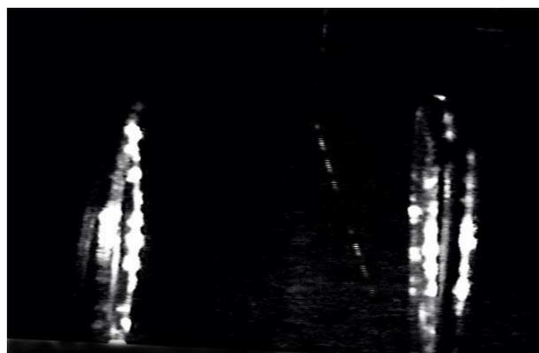
Figure 2. Dust deflection, dust particle being deflected towards the rings are visible on the left hand side
