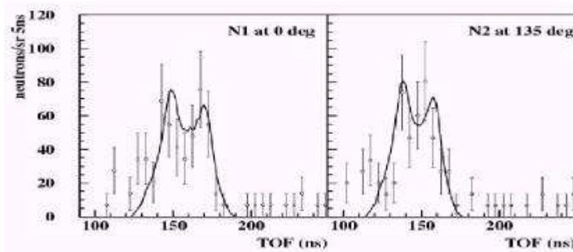
Fig. 2 Neutron emission from a laser irradiated ( $8 \times 10^{18} \text{ W/cm}^2$ )  $\text{D}_2\text{O}$ -spray ( $0^\circ$  - laser propagation; line: calculated signal with  $8 \times 10^{10}$  deuterons (determined from spectral measurement) interacting with the cold target surrounding the laser heated core
