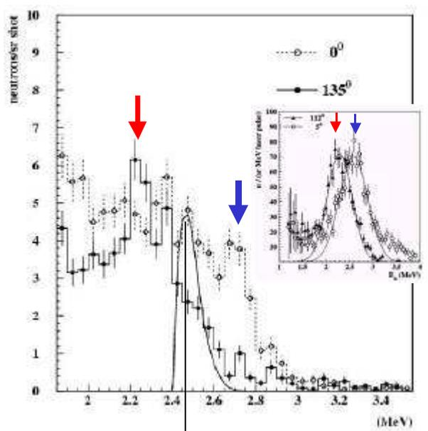
Fig. 1 Measured neutron spectra of the  $0^\circ$  (laser propagation) and  $135^\circ$  n-detector from the  $D_2O$ -droplet target system: the blue- and red-shifted components indicate energetic deuterons moving in the forward (laser) direction, line – calculated n-signal from the droplet neighbors; insert: measured spectral shifts from a flat D-target [5]
