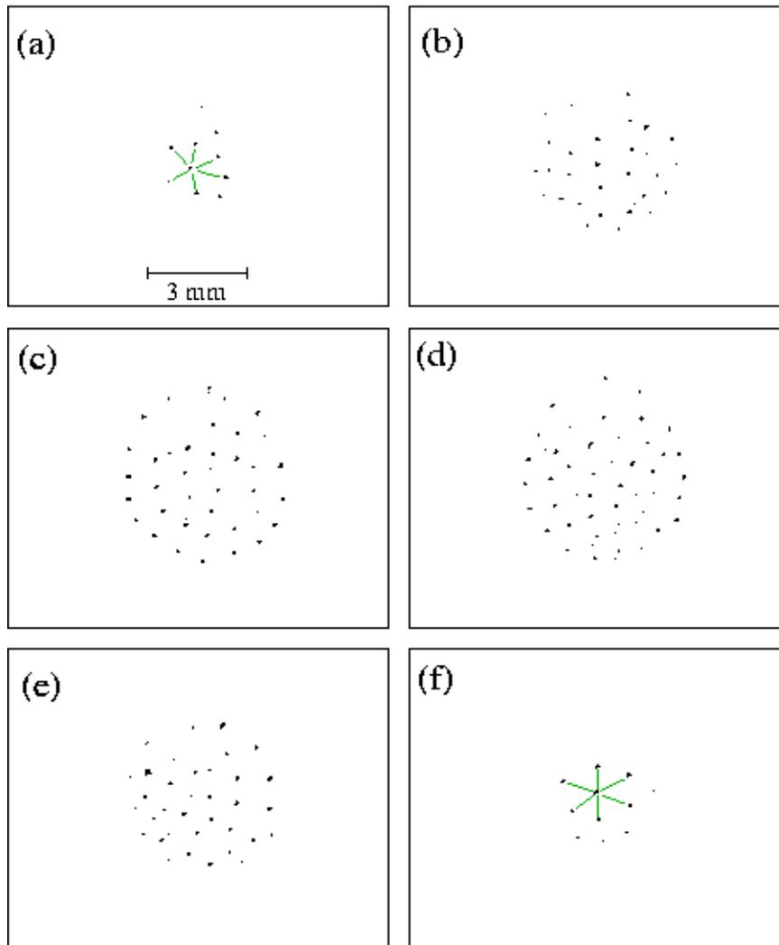
FIG. 2: Series of inverted images of vertical cross sections through the dust cloud. All pictures use the same scaling denoted in (a). The axial distance between subsequent images is about  $880\mu\text{m}$ .
