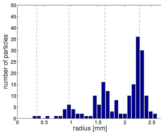
FIG. 3: Radial particle distribution of a dust cloud containing 190 particles. The peaks indicate a concentric shell structure. The dashed lines indicate the average shell radii.
