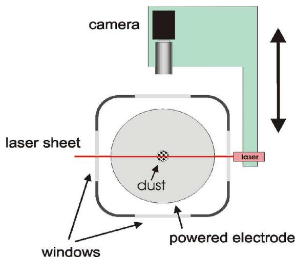
FIG. 1: Experimental setup to obtain 3D particle position. The camera is focused to the plane of the vertically oriented laser fan. Both are mounted on a common positioning system to allow for axial scans.
