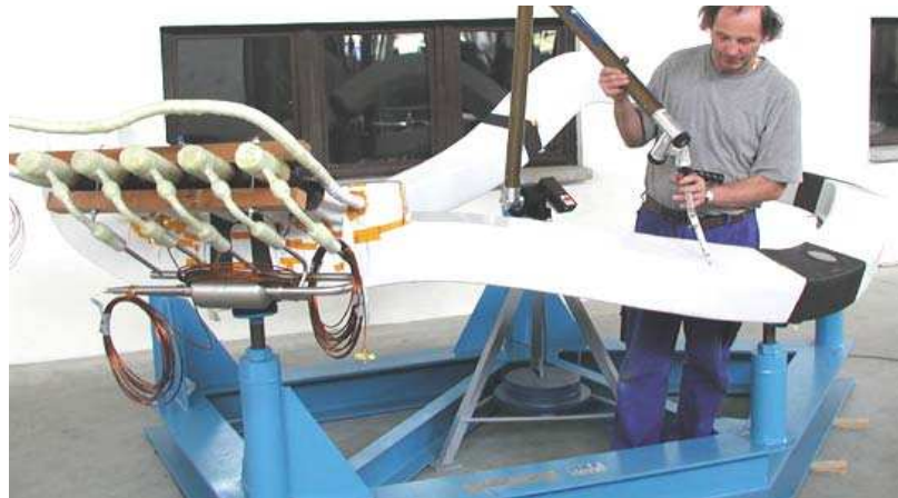
Fig. 1. Dimensional control of a non-planar winding package using a Faro arm
