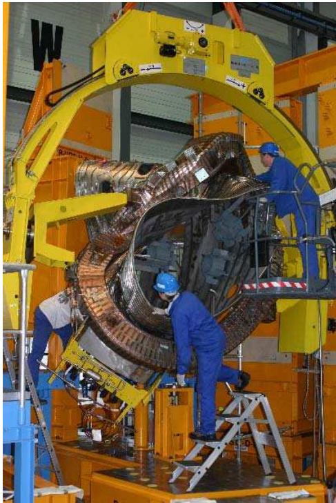
Fig. 2. Stringing of a non-planar coil across the plasma vessel using the coil stringing unit
