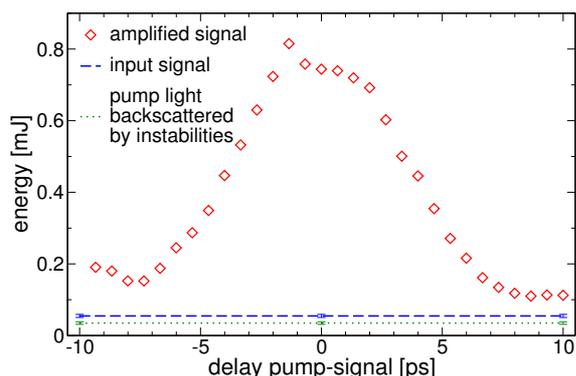
Figure 2: Energy of the amplified signal pulse (diamonds) versus the delay between the pump and signal pulses. The values are averaged over 20 shots.
