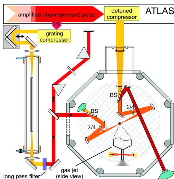
Figure 1: Experimental setup: BS - polarizing beam splitter;  $\lambda/4$  - quarter wave plate.
