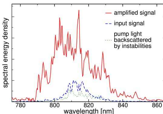
Figure 3: Spectra of the amplified (solid red line) and input pulses (dashed blue line); the delay between the pump and signal pulses is chosen as to maximize the energy gain.
